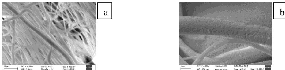
Figure 1: Polymeric fiber (a) and Ceramic fibers (b) produced by Blow-spinning.
